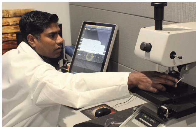
Coating characterizations are analyzed to understand microstructural properties for conformance to specific specifications.
