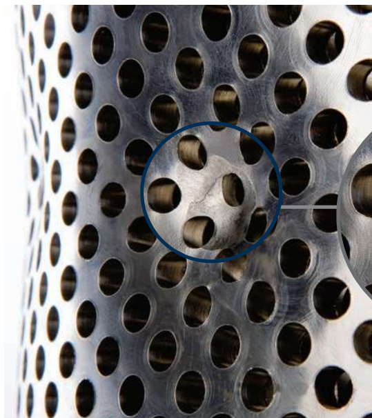
8" "Brick Stopper" with 600 joules impact damage
