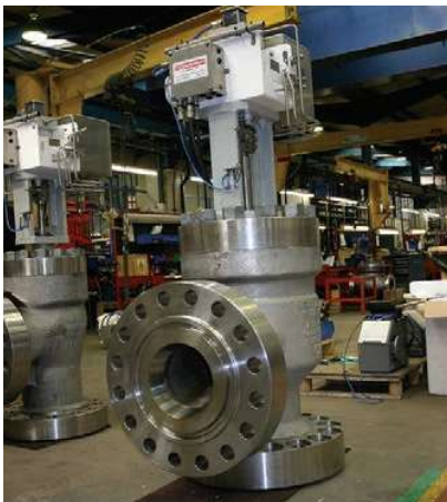
12" ANSI 1500 choke C/W electro-hydraulic actuator
